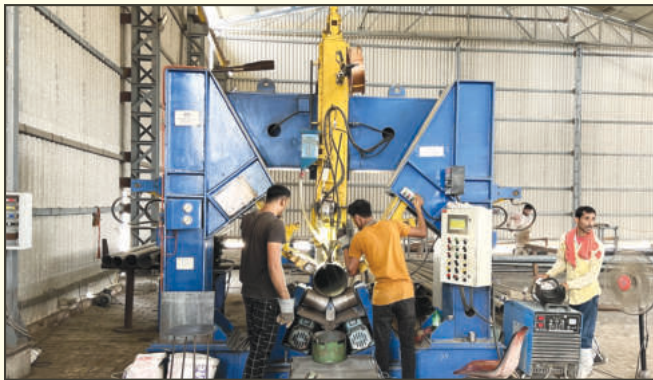
POLE CLOSING WELD
